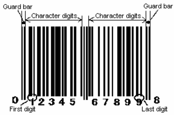
UPC-A print result by the command <D> with subsequent font type selection
