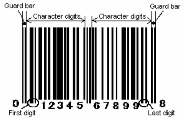
UPC-A print result by the command <BL> with subsequent font type selection
